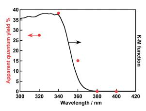
Fig. 3 An action spectrum of water splitting over  $Rh_{0.5}Cr_{1.5}O_3(0.2-wt\%)/AgTaO_3$  and a diffuse reflectance spectrum of  $AgTaO_3$  prepared by a solid state reaction at 1273 K for 15 h without excess Ag.  $Rh_{0.5}Cr_{1.5}O_3$  was loaded by an impregnation method at 623 K for 1 h. Photocatalyst: 0.3 g, reactant solution: distilled water (120 mL), cell: top-irradiation cell with a Pyrex window, light source: 300 W Xe-arc lamp with band-pass filters.
