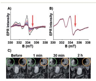
Fig. 3 EPR spectra for the reduction of TMV-6 (2.6 mg mL $^{-1}$ ) with sodium ascorbate (10 equivalents per TEMPO moiety) in the (A) absence and (B) presence of CB[8] (10 equivalents per TEMPO moiety). Data were collected at 10 min intervals over 2 h. (C)  $T_1$  weighted images of CB[8]  $\supset$  TMV-6 (green circle) vs. TMV-6 (orange circle) injected into the thigh muscle of a mouse.
