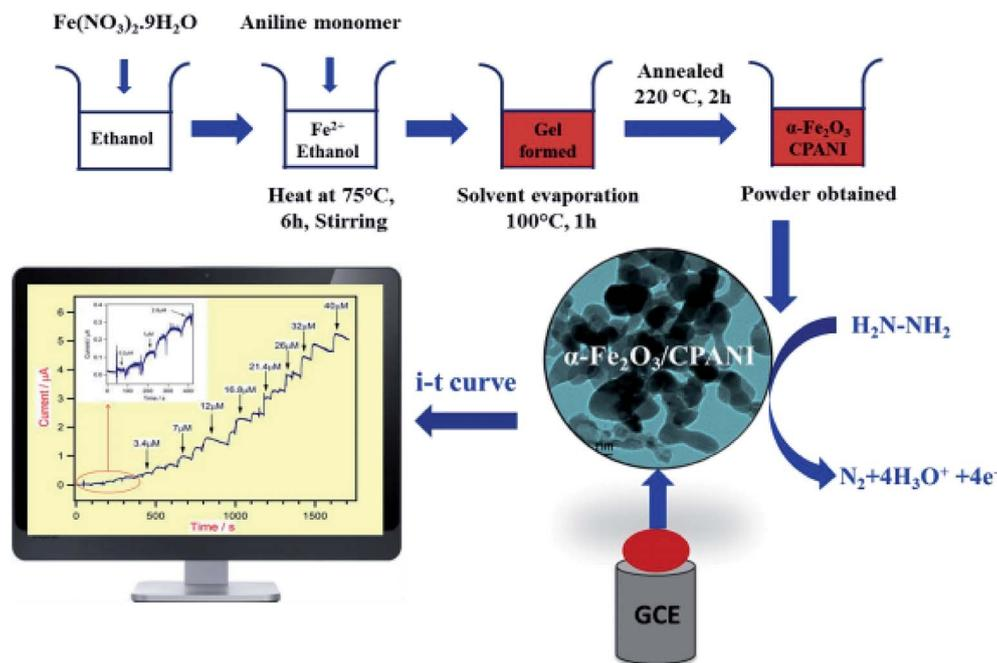
Fig. 6 Schematic representation of the synthesis of the  $\alpha$ -Fe<sub>2</sub>O<sub>3</sub>/CPANI-modified GCE, along with the amperometric detection of hydrazine. Reproduced with permission from ref. 74. Copyright 2016 Elsevier.
