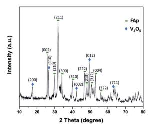
Fig. 2 Powder-XRD spectra of 2.5% V<sub>2</sub>O<sub>5</sub>/FAp catalyst.
