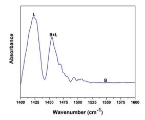
Fig. 5 Pyridine IR spectra of 2.5% V<sub>2</sub>O<sub>5</sub>/FAp catalyst.
