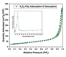
Fig. 3  $N_2$  adsorption–desorption isotherm spectrum of 2.5%  $V_2O_5/$  FAp catalyst.
