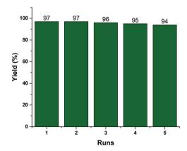
Fig. 6 Recyclability of 2.5% V<sub>2</sub>O<sub>5</sub>/FAp catalyst.
