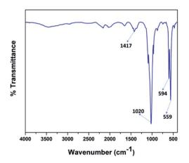
Fig. 4 FT-IR spectra of 2.5% V<sub>2</sub>O<sub>5</sub>/FAp catalyst
