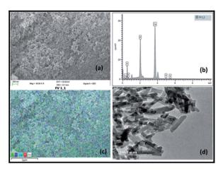
Fig. 1 (a) SEM-micrograph, (b) EDX spectrum, (c) SEM-mapping and (d) TEM-micrograph of 2.5%  $V_2O_5/FAp$  catalyst.
