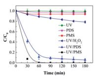
Fig. 1 HA elimination with the UV, PDS, PMS, UV/PDS, UV/PMS, and UV/H $_2$ O $_2$  processes. Conditions: [HA] $_0$  = 15 mg L $^{-1}$ , [PDS] $_0$  = [PMS] $_0$  = [H $_2$ O $_2$ ] $_0$  = 3 mmol L $^{-1}$ , pH $_0$  = 6, 3, and 4 for UV/PDS, UV/PMS, and UV/H $_2$ O $_2$ , respectively.
