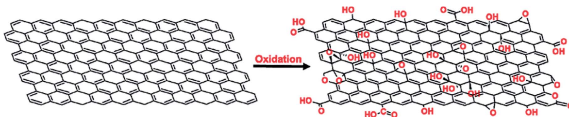
Fig. 2 Oxidation of graphene sheet to form graphene oxide. This figure has been reproduced from ref. 43 with permission from Chem. Rev. , Copyright 2016.
