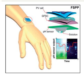
Fig. 8 Schematic representation of fully flexible self-powered wearable pH sensor.<sup>5</sup>
