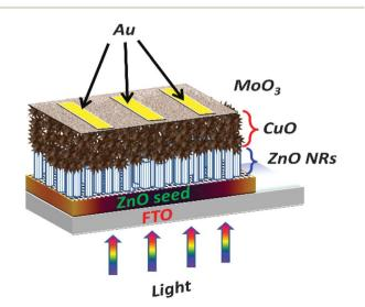
Fig. 1 Schematic design of ZnO/CuO/MoO<sub>3</sub> heterojunction solar cell.
