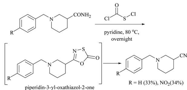
Scheme 5 Chlorocarbonylsulfonyl chloride and pyridine mediated dehydration.
