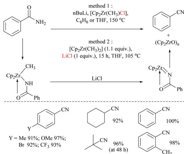
Scheme 19 Zirconium catalyst with LiCl for dehydration.
