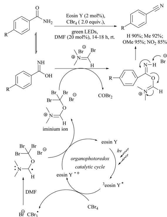
Scheme 53 Organo-photocatalytic dehydration.
