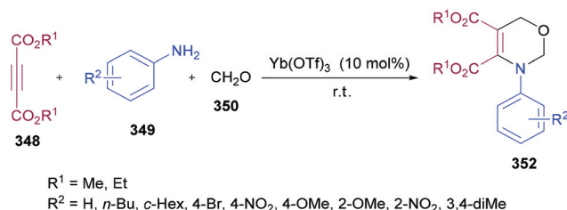
Scheme 89 Ytterbium triflate promoted one-pot three-component synthesis of 3,4,5-trisubstituted-3,6-dihydro-2H-1,3-oxazines.
