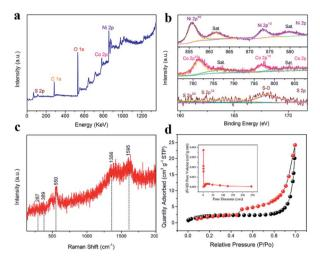
Fig. 3 (a) Clear wide scan XPS spectrum of the NiO/Co $_3$ O $_4$ @C/CoS $_2$  sample; (b) detailed high-resolution XPS spectra of the Ni 2p, Co 2p and S 2p of the NiO/Co $_3$ O $_4$ @C/CoS $_2$  sample; (c) Raman spectrum of the NiO/Co $_3$ O $_4$ @C/CoS $_2$  electrode material; (d) nitrogen adsorption–desorption isotherms and pore-size distribution (inset) of nickel foam coated with the NiO/Co $_3$ O $_4$ @C/CoS $_2$  sample.
