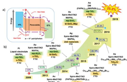
Fig. 3 (a) Schematic diagram and energy band of interfaces among the electron transport layer (ETL)/perovskite/hole transport layer (HTL). (b) The representative progress of ETLs in the *n-i-p* architecture.
