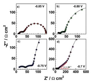
Fig. 6 Impedance spectra of a PSC with FTO/compact  $TiO_2$ /mesoporous  $TiO_2$ (MAPbl<sub>3</sub>)/spiro-OMeTAD/Au structure using mesoporous  $TiO_2$ ( $\sim$ 20 nm diameter, 800 nm thickness) film as a photo-anode filled with MAPbl<sub>3</sub>, obtained under dark conditions with different bias: (a–d) Nyquist plots (-0.85, -0.8, -0.75, and -0.7 V, respectively).
