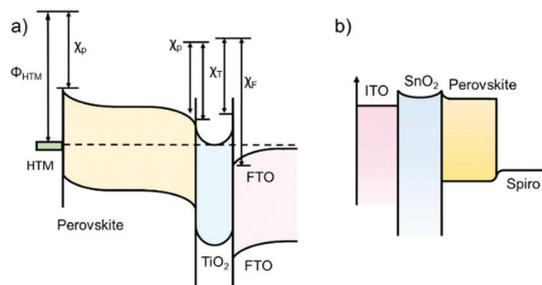
**Fig. 8** (a) Energy-band diagram deduced from the vacuum energy levels.  $\chi_p$ ,  $\chi_T$  and  $\chi_F$  represent the electron affinities of the perovskite, TiO<sub>2</sub> and FTO layers, respectively, and  $\Phi_{\text{HTM}}$  represents the work function of the HTM layer. (Modified from ref. 78.) (b) The simplified energy-band diagram for the planar structured PSC.
