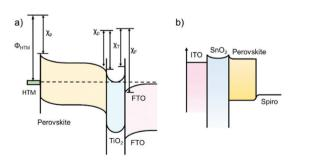
Fig. 8 (a) Energy-band diagram deduced from the vacuum energy levels.  $\chi_{P},~\chi_{T}$  and  $\chi_{F}$  represent the electron affinities of the perovskite, TiO  $_{2}$  and FTO layers, respectively, and  $\Phi_{\mathrm{HTM}}$  represents the work function of the HTM layer. (Modified from ref. 78.) (b) The simplified energy-band diagram for the planar structured PSC
