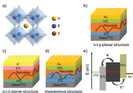
**Fig. 1** (a) Illustration of a crystalline structure of perovskite  $ABX_3$ , A:  $MA^+$  or  $FA^+$  cation, B:  $Pb^{2+}$  cation, X:  $Cl^-$ ,  $Br^-$  or  $I^-$  anion. Typical perovskite solar cells with (b) n–i–p structure, (c) p–i–n structure, and (d) mesoporous structure. (e) Energy level scheme for the transporting direction of electron and hole carriers in n–i–p perovskite solar cells.
