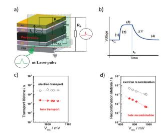
Fig. 9 (a and b) The working scheme of transient photovoltage/photocurrent decay measurement. (b) Shows transient photocurrent decay data for an example device. (c) Transport lifetime and (d) recombination lifetime results from using bi-exponential fitting of the transient photocurrent decay and transient photovoltage decay, respectively.
