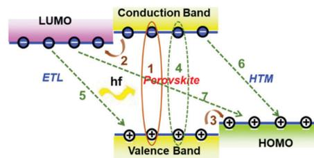
Fig. 4 Diagram for charge transfer, collection and recombination of planar PSCs with a structure of ITO/ETL/MAPbI<sub>3</sub>/HTM/Au. Photon exciton (1), charge transfer (2 and 3), collection and recombination (4, 5, 6, 7) steps take place at the interfaces. The thick green and thin red arrows respectively indicate the processes desirable for energy conversion and those associated with losses. hf, photon energy.
