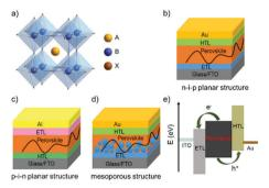
Fig. 1 (a) Illustration of a crystalline structure of perovskite ABX<sub>3</sub>, A: MA<sup>+</sup> or FA<sup>+</sup> cation, B: Pb<sup>2+</sup> cation, X: Cl<sup>-</sup>, Br<sup>-</sup> or I<sup>-</sup> anion. Typical perovskite solar cells with (b) n-i-p structure, (c) p-i-n structure, and (d) mesoporous structure. (e) Energy level scheme for the transporting direction of electron and hole carriers in n-i-p perovskite solar cells
