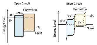
Fig. 10 Electron energy levels at open circuit (left) for the transient photovoltage decay measurement and at short circuit (right) for the transient photocurrent decay measurement on a PSC using SnO2 and spiro-OMeTAD as ETL and HTL. The dotted lines indicate the Fermi level of electrons and holes in the perovskite layer.
