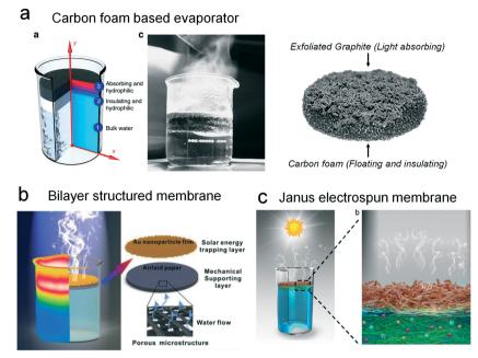
Fig. 3 Typical evaporators in direct contact mode. (a) Carbon foam-based solar steam generator.<sup>30</sup> (b) Janus evaporator that is composed of gold nanoparticles and air-laid paper.<sup>31</sup> (c) Salt rejecting evaporator with a hydrophobic/hydrophilic binary structure.<sup>32</sup>
