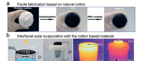
Fig. 12 Low-cost cotton based solar evaporator. (a) The rapid fabrication of light absorbing cotton. (b) The oil lamp inspired solar evaporator exhibits an obvious interfacial heating ability.<sup>70</sup>
