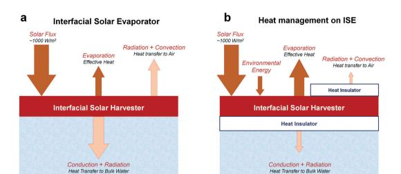
Fig. 9 The heat transfer during the interfacial solar evaporation (ISE). (a) The conventional evaporator and (b) the novel evaporation system with precise heat management.
