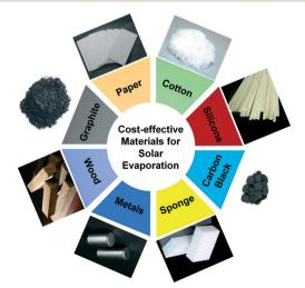
Fig. 11 The cost-efficient materials that are used in solar evaporation, including low price photothermal materials (carbon black and graphite), cellulose-based hydrophilic substrates (paper and cotton), and effective floating supports (wood and sponge).
