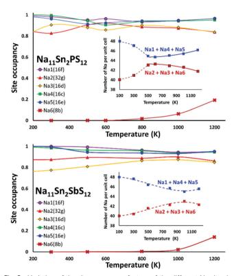
Fig. 8 Variation of the site occupancy factors of the different Na sites in Na<sub>11</sub>Sn<sub>2</sub>PS<sub>12</sub> (top) or Na<sub>11</sub>Sn<sub>2</sub>SbS<sub>12</sub> (bottom) over the temperature range 300 K to 1200 K. The respective insets display the same data as number of Na on the two groups of sites, i.e. the Na2-Na3-Na6 site cluster and the Na1-Na4-Na5 group of interconnecting sites.
