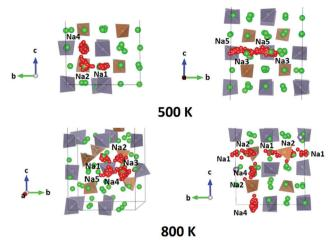
Fig. 7 Typical Na<sup>+</sup> ion trajectories in Na<sub>11</sub>Sn<sub>2</sub>PS<sub>12</sub> at T = 500 K (top row) and 800 K (bottom row). Diffusion occurs in all three dimensions. Grey (brown) tetrahedra represent SnS<sub>4</sub> (PS<sub>4</sub>). Spheres represent Na sites, among which those marked in red correspond to Na sites along the selected trajectories.
