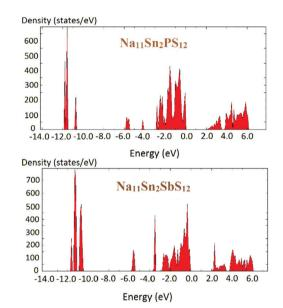
Density of states of Na<sub>11</sub>Sn<sub>2</sub>PS<sub>12</sub> and Na<sub>11</sub>Sn<sub>2</sub>SbS<sub>12</sub>.
