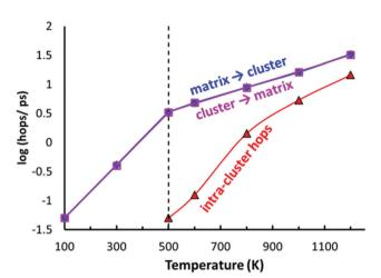
Fig. 10 Temperature dependences of the site-specific hop frequencies in AIMD simulations of  $Na_{11}Sn_2PS_{12}$ . Hops are classified into hops from the  $(Na2)_4(Na3)_2Na6$  site cluster to the interconnecting "matrix sites" Na1, Na4 or Na5 (magenta open squares), *vice versa* (blue filled diamonds), or intra-cluster rearrangements within the vacancy-rich  $(Na2)_4(Na3)_2Na6$  cluster (red triangles). The broken vertical line marks the onset of PS<sub>4</sub> rotational disorder above 500 K.
