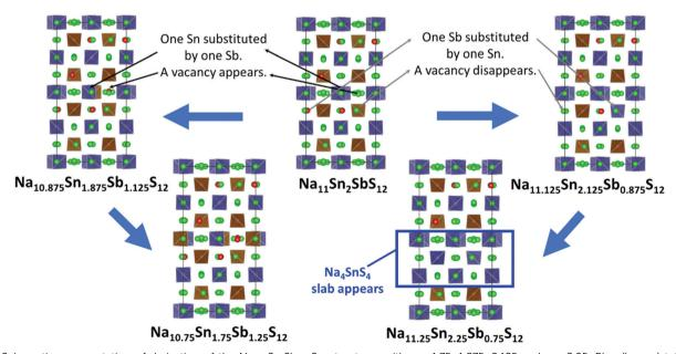
Fig. 4 Schematic representation of derivation of the  $Na_{9+x}Sn_xSb_{3-x}Sl_2$  structures with x = 1.75, 1.875, 2.125 and x = 2.25. Blue (brown) tetrahedra  $represent SnS4 (SbS4), green spheres occupied Na sites. Na vacancies are marked in red. For Na_{11.25}Sn_{2.25}Sb_{0.75}S_{12} the lowest energy structure contains a property of the contains a site of the$ slab of Na<sub>4</sub>SnS<sub>4</sub> composition marked in blue.
