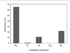
Fig. 3 Typical uncertainty budget for dynamic mass flow method, using 30 nm Au NP as an example.  $N_{\rm NP}$  is the number of particles detected in time scan,  $D_{\rm f}$  is sample dilution factor, TE is the transport efficiency,  $Q_{\rm sam}$  is the sample mass flow and  $B_{\rm var}$  is the batch-to-batch variability.
