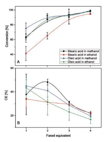
Fig. 7 (A) Degree of the electrochemical decarboxylation of stearic acid and oleic acid in MeOH and EtOH as a function of the applied charge. (B) The faradaic efficiency *vs.* the flown charge. <sup>105</sup> Reprinted from ref. 105, Copyright (2015), with permission from John Wiley *&* Sons Ltd.
