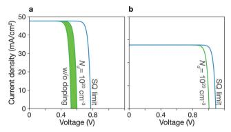
Fig. 7 Current-voltage simulation. J-V curves for CZTSe (a) and AZTSe (b) solar cells based on the properties of the bulk absorber materials and not including interfacial processes. Green lines represent the TLCs with various doping concentrations up to  $10^{20}$  cm $^{-3}$ . The SQ limit is shown in the blue curve.
