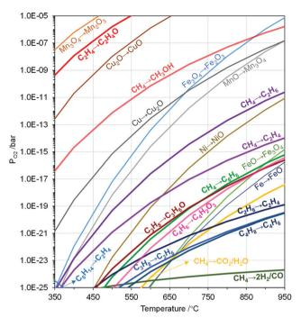
Fig. 8 Modified Ellingham diagram of metal oxide redox and POx reactions.  $MeO_x \rightarrow MeO_y$  and hydrocarbons POx reactions correspond to the  $P_{O_2}$  when  $\Delta G = 0$ . Reactions in pathways of  $MeO_x \rightarrow MeO_y$  and hydrocarbons POx are given in Table 2.
