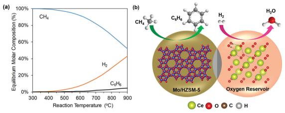
Fig. 11 (a) Equilibrium product composition of CH<sub>4</sub> DHA as a function of reaction temperature. (b) A potential configuration of methane CL-DHA process (the air regeneration step is not shown).<sup>240</sup>
