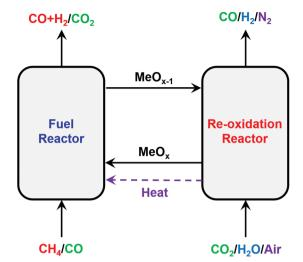
Fig. 10 Schematic and reaction schemes of different CL cycles for conversion of  $CH_4$  to synthesis gas.
