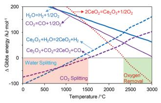
Fig. 4 Ellingham diagram of thermal and chemical looping water and CO<sub>2</sub> splitting. Light green and red regions represent thermodynamically spontaneous ( $K \ge 1$ ) reduction and oxidation reactions, respectively. In practice, a reaction would occur when K < 1.
