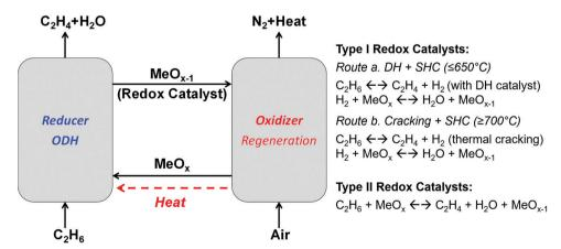
Fig. 12 Schematic of CL-ODH, redox catalyst types, and reaction schemes. Ethane is used as an example for light alkanes for illustration purpose.
