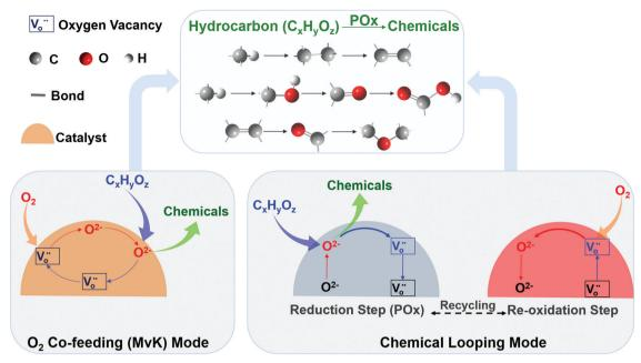
Fig. 16 Comparison of  $O_2$  co-feeding (MvK) and chemical looping modes for partial oxidations and their applications on conversions of hydrocarbon to chemicals (transformation between alkane, alkene, alcohol, aldehyde, ketone, acid, and aromatics).
