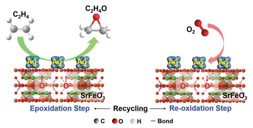
Fig. 13 The reaction mechanism of chemical looping epoxidation using a silver-modified  $SrFeO_{3-\delta}$  redox catalyst
