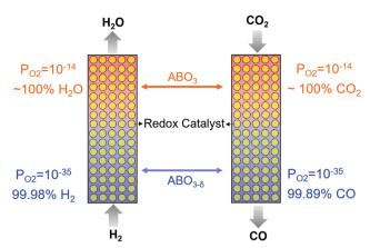
Fig. 7 RWGS in a counter-currently operated two-step chemical looping scheme using ABO<sub>3</sub> perovskite as a redox catalyst at 500 °C.
