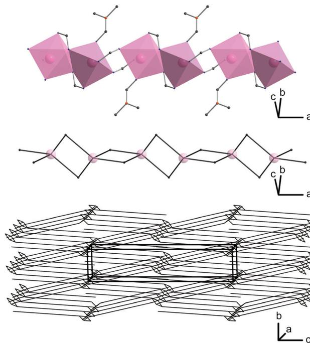
Fig. 4 Octahedrally coordinated cadmium(II) in 2 forming chains along the *a* axis (top), its transformed 4<sup>2</sup>-net (middle) and the resulting final dmd net-type (bottom).
