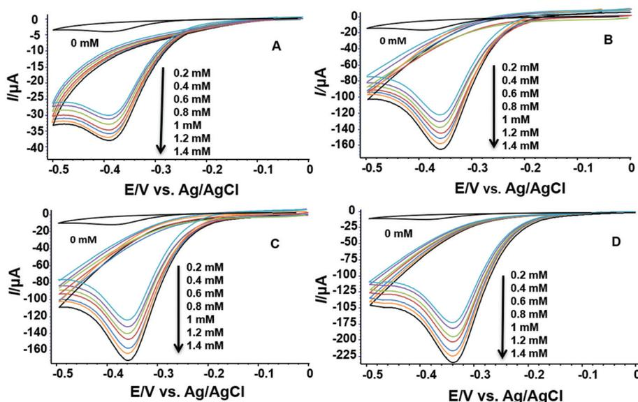
Fig. 5 Electrochemical reduction of  $\text{H}_2\text{O}_2$  (various concentrations) on (A) bare GC electrode, (B) GC electrode modified with  $\text{H}_2\text{L}$ , (C) GC electrode modified with compound **1**, and (D) GC electrode modified with compound **2**.
