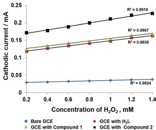
Fig. 7 Relationship between cathodic current and H<sub>2</sub>O<sub>2</sub> concentration in the four cases mentioned above (Fig. 5).
