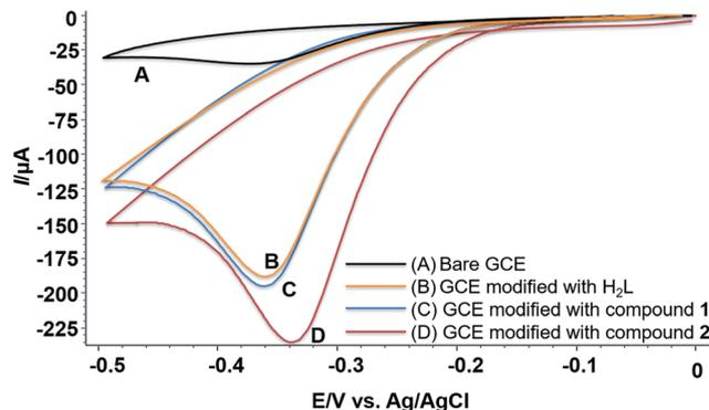
Fig. 6 Voltammetric response of (A) bare GC electrode; (B) GC electrode modified with  $\text{H}_2\text{L}$ , (C) GC electrode modified with compound **1**, and (D) GC electrode modified with compound **2** in  $1.4 \text{ mM H}_2\text{O}_2$ .
