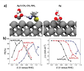
Fig. 31 (a) Chemisorbed CO<sub>2</sub> on cysteamine-functionalized (left) and on cysteamine-free (right) Ag(111) surface. Only the water molecules directly forming hydrogen bond (slashed line) are shown. The colors are: Ag in silver, C in gray, O in red, N in blue, S in yellow, and H in white. (b) Influence of the alkyl chain length on  $CO_2RR$  in terms of  $FE_{CO}$  (left) or  $j_{CO}$  (right) vs. potential. Reproduced with permission from ref. 419. Copyright 2018 American Chemical Society
