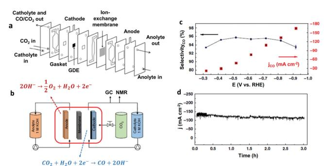
Fig. 11 (a) Cross-sectional view of the CO<sub>2</sub> electrolyzer flow cell and (b) general scheme of the entire experimental set-up used in ref. 186. (c) Current density (right) and selectivity for CO production (left) as a function of the potential, and (d) bulk electrolysis at a fixed potential (E = -0.72 V vs. RHE) for 37@carbon black deposited onto a carbon paper as cathodic material, in 1 M KOH. Adapted with permission from ref. 186. Copyright 2019, Nature Publishing Group
