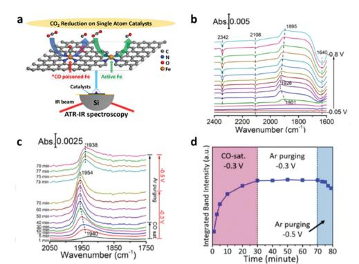
Fig. 23 (a) Scheme of the setup. (b) Real-time ATR-IR spectra recorded while stepping the potential of the Fe-N-C-loaded Au/Si prism in the CO<sub>2</sub>-saturated 0.5 M KHCO<sub>3</sub>. (c) Real-time IR spectra and (d) the evolution of the integrated \*CO band intensity when switching the CO/Ar atmosphere and potential. IR references were taken at 0 V for panel (b) and 0.1 V for panel and (c). Adapted with permission from ref. 339. Copyright 2019 American Chemical Society.
