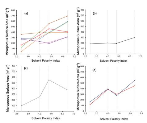
Fig. 2 Plot of the microporous surface area of CMP networks against the polarity index of the reaction solvent. (a) CMP networks 1, 2, 3, 5, 6, 7, and 8 key: CMP-1 – blue, CMP-2 – orange, CMP-3 – pink, CMP-5 – purple, CMP-6 – green, CMP-7 – red, CMP-8 – brown. (b) CMP network 4 (c) CMP network 9 (d) CMP networks 10–11 against the polarity index of the reaction solvent. (Region of the reaction solvent) Region of the reaction solvent (Park No. 1) Place (Park No. 1) P
