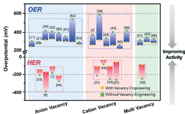
Fig. 8 Trend of the performance of recent vacancy-engineered electrocatalysts.
