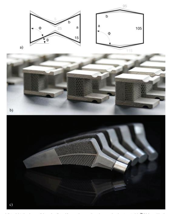
Fig. 4 (a) From left to right, the shapes of the unit cell used for creating auxetic and conventional metamaterials.<sup>79</sup> (b) A combination of the positive and negative values of the Poisson's ratio could be used to create compression around the periphery of hip stems (c).<sup>79</sup>
