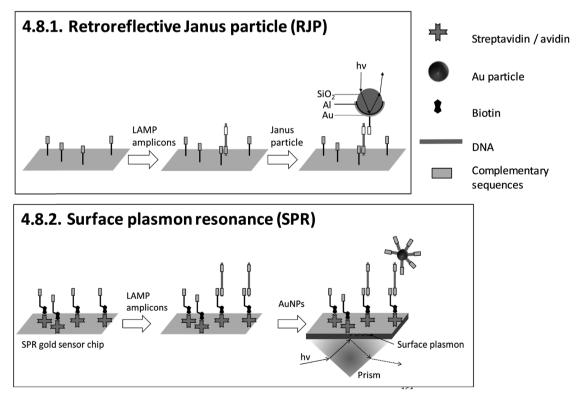
Fig. 10 Schematic illustrations of 4.8.1. retroreflective Janus particle (RJP)<sup>164</sup> and 4.8.2. surface plasmon resonance (SPR)<sup>166</sup> (redrawn according to the references).
