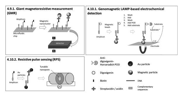
Fig. 11 Schematic illustrations of 4.9.1. giant magnetoresistive (GMR) measurement,<sup>170</sup> 4.10.1. genomagnetic LAMP-based electrochemical detection<sup>171</sup> and 4.10.2. resistive pulse sensing<sup>173</sup> (redrawn according to the references).
