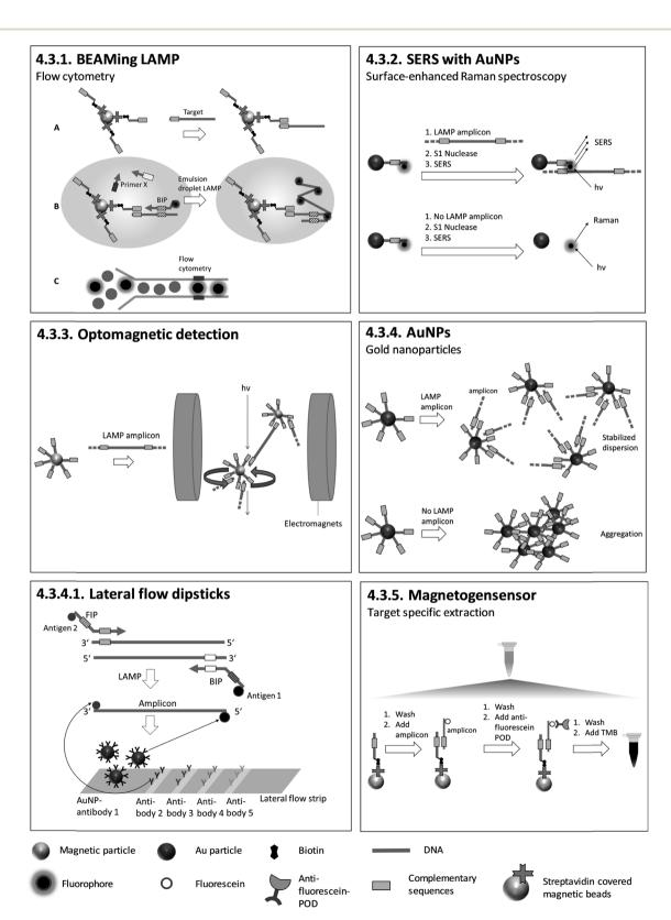
Fig. 7 Schematic illustrations of 4.3.1. BEAMing LAMP, 107 4.3.2. surface-enhanced Raman spectroscopy (SERS) with AuNPs, 111 4.3.3. optomagnetic detection,<sup>112</sup> 4.3.4. AuNPs,<sup>115</sup> 4.3.4.1. lateral flow dipsticks<sup>125</sup> and 4.3.5. magnetogenosensor<sup>148</sup> (redrawn according to the references).
