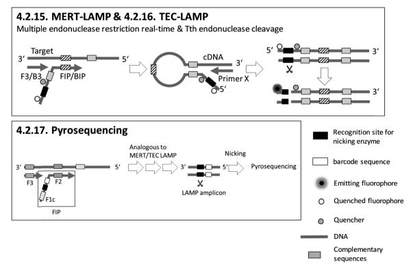
Fig. 6 Schematic illustrations of 4.2.15. MERT-LAMP,<sup>103</sup> 4.2.16. TEC-LAMP<sup>105</sup> and 4.2.17. pyrosequencing<sup>106</sup> (redrawn according to the references)
