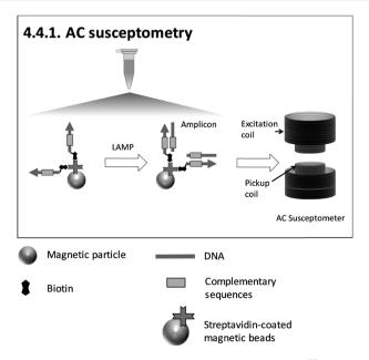
Fig. 8 Schematic illustration of 4.4.1. AC susceptometry<sup>150</sup> (redrawn according to the references).
