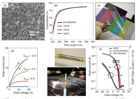
Fig. 4 Polymer TFTs fabricated by Fujisaki et al. on optically transparent heat-resistant nanocellulose paper (nanopaper). The TFTs have a channel length of 10  $\mu$ m and excellent electrical performance, including a carrier mobility of 1.3 cm<sup>2</sup> V<sup>-1</sup> s<sup>-1</sup>, an on/off ratio of 10<sup>8</sup> and a subthreshold slope of 0.84 V per decade. Reprinted with permission. 36 Copyright 2014, Wiley-VCH.
