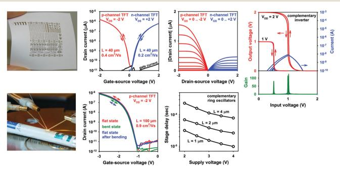
Fig. 7 Low-voltage organic TFTs and complementary circuits fabricated on commercially available cleanroom paper (top) and on a banknote (bottom).46,47
