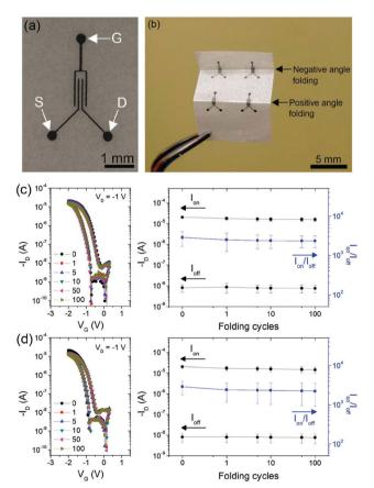
Fig. 5 Electrolyte-gated organic TFTs fabricated by Hyun *et al.* on glassine paper in a side-gate architecture using screen-printed graphene source/drain contacts and gate electrodes, aerosol-jet-printed poly(3-hexylthiophene) and a drop-cast ion-gel electrolyte. The TFTs have a carrier mobility of  $0.14~\rm cm^2~V^{-1}~s^{-1}$ , an on/off ratio of about  $10^3$  and excellent bending stability. Reprinted with permission. <sup>39</sup> Copyright 2015, Wiley-VCH.
