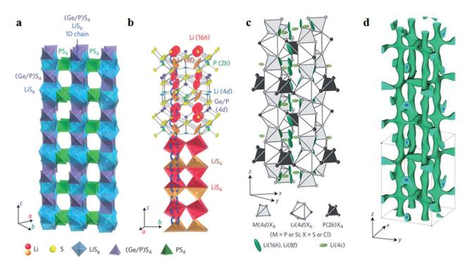
Fig. 4 (a) Framework structure of LGPS; (b) Li $^+$  conduction pathways in LGPS; (c) crystal structure of Li $_{9.54}$ Si $_{1.74}$ P $_{1.44}$ Si $_{1.7}$ Cl $_{0.3}$ ; (d) nuclear distributions of Li atoms in Li<sub>9.54</sub>Si<sub>1.74</sub>P<sub>1.44</sub>S<sub>11.7</sub>Cl<sub>0.3</sub> at 25 °C. Reproduced with permission.<sup>37,38</sup> Copyright© (2011, 2016), Springer Nature.
