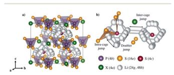
Fig. 6 (a) Crystal structures of  $\text{Li}_6\text{PS}_5\text{X}$  with X = Cl, Br, and I. (b) Lithium ion transport mechanism. Reproduced with permission. Copyright 2017, American Chemical Society.
