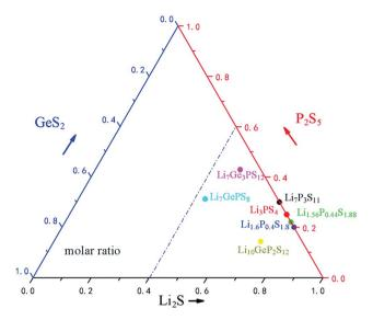
Fig. 5 Li<sub>2</sub>S-P<sub>2</sub>S<sub>5</sub>-GeS<sub>2</sub> ternary phase diagrams.
