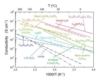
Fig. 7 Thermal evolution of ionic conductivity for different types of solid electrolytes. Reprinted with permission.<sup>81</sup> Copyright© 2018, Royal Society of Chemistry.
