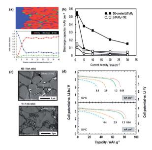
Fig. 12 (a) Volume fractions of respective materials along the electrode thickness; (b) electrochemical performance of S-SE-coated  $LiCoO_2$  and  $LiCoO_2 + S-SE$ ; (c) S-SE-coated  $LiCoO_2$  particles with different grain sizes; (d) electrochemical performances of different cathode compositions. Reproduced with permission.<sup>109</sup> Copyright© 2017, Royal Society of Chemistry.
