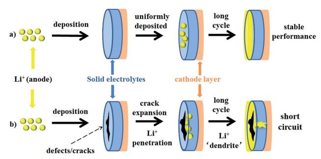
Fig. 22 Schematic diagrams of the mechanism of penetration of Li-ions into solid electrolytes. (a) Li-ions are uniformly deposited on the surface of the defect-free electrolyte; (b) penetration of Li-ions into the solid electrolyte layer forming 'dendrites' through defects, causing short circuit. Produced with permission. Copyright@ 2017, John Wiley and Sons.
