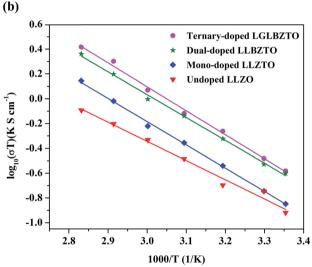
Fig. 4 (a) AC impedance plot of the garnet-type ternary-doped LGLBZTO  $Li_{6.65}Ga_{0.05}La_{2.95}Ba_{0.05}Zr_{1.75}Ta_{0.25}O_{12}.$  The inset shows partially enlarged graph at the high frequency region. The equivalent circuit is used to fit the curve. (b) Arrhenius plot of the undoped LLZO, mono-doped LLZTO, dual-doped LLBZTO, and ternary-doped LGLBZTO.
