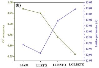
Fig. 5 Comparison plot for (a) density and total ionic conductivity at room temperature and Li occupancy ratio at  $96h_{\rm Li2}/24d_{\rm Li1}$ . (b)  $\rm O^{2-}$  occupancy with lattice parameters of the undoped LLZO, monodoped LLZTO, dual-doped LLBZTO, and ternary-doped LGLBZTO. The total ionic conductivity and density increase, whereas the Li occupancy ratio at  $96h_{\rm Li2}/24d_{\rm Li1}$  decreases with multi-ion doping into the garnet.
