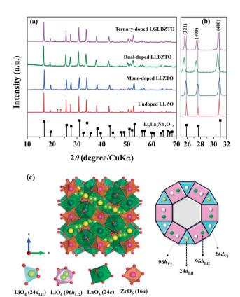
Fig. 1 (a) XRD patterns and (b) peak shift of the undoped LLZO, monodoped LLZTO, dual-doped LLBZTO, and ternary-doped LGLBZTO in the range of  $25^{\circ}-32^{\circ}$ . (c) Crystal structure of cubic LLZO with the connectivity pattern of tetrahedral-24d $_{\rm Li1}$  and 96h $_{\rm Li2}$  cages projected on two dimensions.
