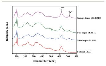
Fig. 2 Raman spectra of the undoped LLZO, mono-doped LLZTO, dual-doped LLBZTO, and ternary-doped LGLBZTO in the range of 50–800 cm<sup>-1</sup>.
