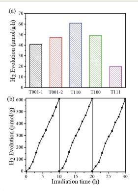
Fig. 4 (a) Photocatalytic hydrogen production using NH<sub>2</sub>-MIL-125(Ti) with different morphologies. (b) Recycling tests using T110.
