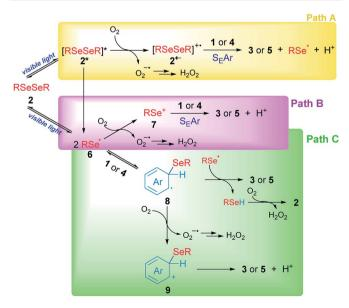
Scheme 5 Proposed mechanisms for the synthesis of selenium compounds.
