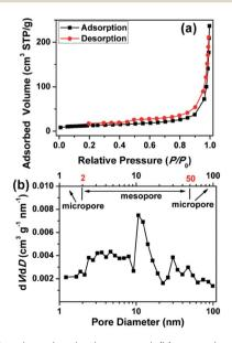
Fig. 3 (a) N<sub>2</sub> adsorption isotherms and (b) pore size distributions calculated by BJH method of the HWGF.
