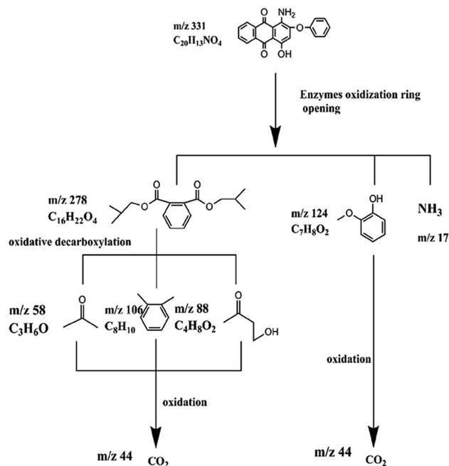
Fig. 11 Degradation pathway analysis of Disperse Red 3B.
