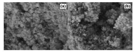
Fig. 5 The FE-SEM images of Pd@MTiO<sub>2</sub> material at high (a) and low (b) resolutions
