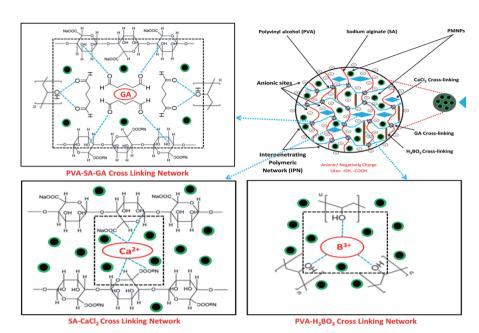
Fig. 3 Conceptual possible cross-linking networks of  $SA-CaCl_2$ ,  $PVA-H_3BO_3$  and PVA-SA-GA during the fabrication of bio-magnetic membrane capsules (BMMCs). (Reproduced from Ali *et al.*<sup>24</sup> Copyright@2019, with permission from Elsevier Ltd.)
