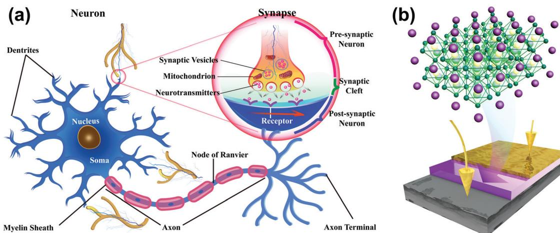
Fig. 1 Schematics of (a) a biological neuron and (b) a two-terminal artificial synapse based on HP.
