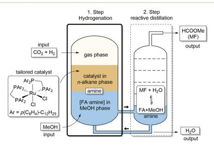
Fig. 1 Integrated process for catalytic hydrogenation and reactive distillation for production of methyl formate (MF) from CO<sub>2</sub>, H<sub>2</sub> and MeOH.
