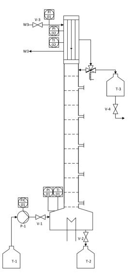
Schematic depiction of the rectification setup used for the reactive distillation of the MeOH/FA/1,2-DMI mixture.
