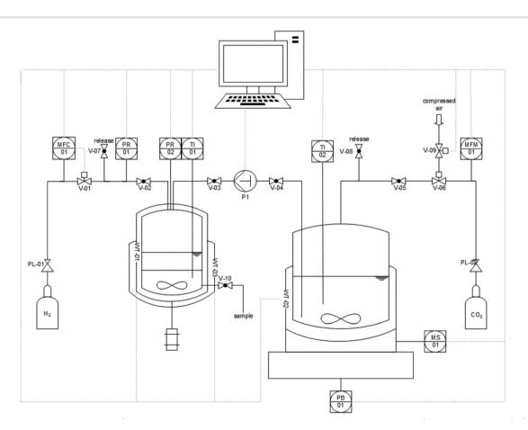
Fig. 5 Schematic depiction of the semi-continuous operated set-up with a 100 mL autoclave for hydrogenation (left) and a 900 mL autoclave as reservoir for CO<sub>2</sub> pre-saturated solutions of 1,2-DMI in methanol (right).
