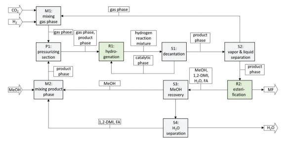
Fig. 8 Block flow diagram of a continuous process for the production of MF from CO<sub>2</sub>. Ri = Reaction units, Si = separation units, Mi = mixing units.
