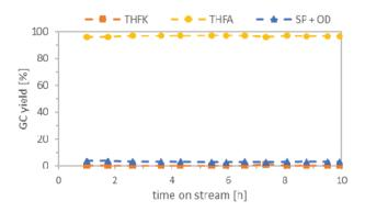
Fig. 7 Continuous Flow Hydrogenation of a FFA (0.25 mol  $L^{-1}$ ) solution in cyclohexane. Conditions: Catalyst bed: 1 g Ru/C, 50 °C, substrate flowrate: 1 mL min<sup>-1</sup>, hydrogen flowrate: 37 mL<sub>N</sub> min<sup>-1</sup>, pressure: 80 bar, WHSV = 2 h<sup>-1</sup>.
