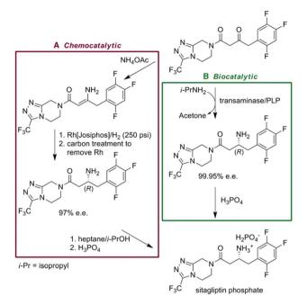
Fig. 5 Comparison of Merck's chemocatalytic and Biocatalytic syntheses for their antidiabetic drug Sitagliptin. Reprinted with permission from AAAS. 106
