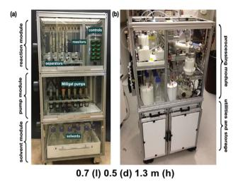
Fig. 10 Units designed for the pharmacy on demand initiative, phase two. Reprinted with permission from Wiley  $\vartheta$  Sons. <sup>180</sup>
