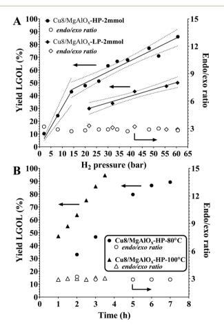
Fig. 2 (A) Effect of the  $H_2$  pressure on the LGOL yield and its *endo/exo* ratio for the Cu8/MgAlO<sub>x</sub>-HP and Cu8/MgAlO<sub>x</sub>-LP catalysed Cyrene to LGOL conversion at 333 K for 18 h (B) influence of the temperature (353 & 373 K) on the Cyrene to LGOL reaction with the Cu8/MgAlO<sub>x</sub>-HP catalyst. Batch reactor. All batch experiments were conducted with 2 mmol Cyrene in 5 mL water (~4.9 wt%), 25 mg catalyst and 60 bar  $H_2$ .
