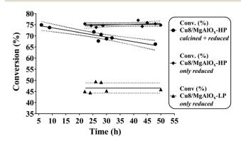
Fig. 7 Comparative activity of "oxidized and reduced" and "sole reduced" Cu8/MgAlO $_x$ -HP in flow (353 K, 60 bar H $_2$ , 1 wt% Cyrene in H $_2$ O). Flow conditions: Cyrene/H $_2$ O solution: 0.03 mL min $^{-1}$ , H $_2$  gas: 20 mL min $^{-1}$ .
