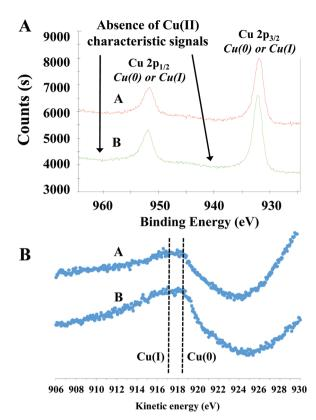
Fig. 4 (A) X-ray photoelectron spectroscopy (XPS) data of Cu8/ MgAlO<sub>x</sub>-HP (scan A) and Cu8/MgAlO<sub>x</sub>-LP (scan B); (B) Auger LMM spectra of Cu8/MgAlO<sub>x</sub>-HP (scan A) and Cu8/MgAlO<sub>x</sub>-LP (scan B).
