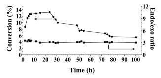
Fig. 8 Activity of reduced Cu8/MgAlOx-HP in flow (353 K, 60 bar H<sub>2</sub>, 5 wt% Cyrene in H<sub>2</sub>O). Flow conditions: Cyrene/H<sub>2</sub>O solution: 0.03  $mL min^{-1}$ ,  $H_2$  gas: 20  $mL min^{-1}$ .
