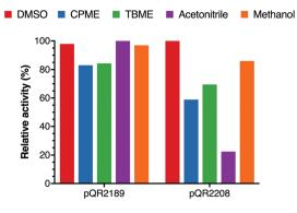
Fig. 5 Effect on yield of 18b with various co-solvents (10% final concentration). The reaction conditions used were the same as those indicated in Fig. 4, all reactions were performed in triplicate and standard deviations were <8%.
