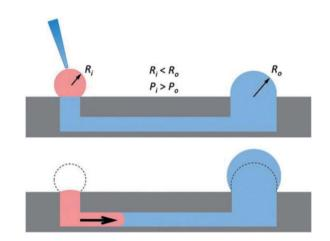
Fig. 4 Diagram showing the mechanism of passive pumping. Passive pumping depends on the radius of each droplet. The pressure from a small droplet of radius  $R_{\rm i}$  will be larger than the pressure from a large droplet of radius  $R_{\rm o}$  based on Laplace's law. (Adapted from ref. 57 with permission from The Royal Society of Chemistry).
