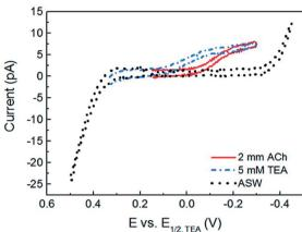
Fig. 5 (A) Photograph and (B) scanning electron micrograph of a nanopipette prepared by a laser-pulled capillary. (C) Cyclic voltammogram of 2 mM acetylcholine (ACh), tetraethylammonium (TEA), and artificial seawater (ASW). TEA was used as an internal standard and ASW was the solvent (background signal). Adapted with permission from Colombo et al.<sup>81</sup>
