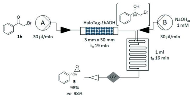
**Fig. 5** Two-step chemo-enzymatic synthesis of (*S*)-2-phenyloxirane **5**. Pump A loading the packed-bed reactor containing immobilized HaloTag-LbADH: flow rate 30 μl min<sup>-1</sup>, ketone **1h** (50 mM), NADPH (0.5 mM), 2-propanol (10 vol%), THF (30 vol%), KPi 50 mM (pH 7.0), MgCl<sub>2</sub>·H<sub>2</sub>O (1 mM). Pump B loading the glass microreactor (2 inputs, 1 ml): flow rate 30 μl min<sup>-1</sup>, NaOH (1 mM, pH 13). Conversion determined by <sup>1</sup>H-NMR.
