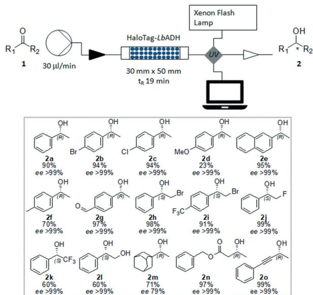
**Fig. 4** Asymmetric reduction of ketones by using the immobilized HaloTag-LbADH in flow. Reaction conditions: ketones **1a–1o** (50 mM), NADPH (0.5 mM), 2-propanol (10 vol%), THF (30 vol%), KPi 50 mM (pH 7.0), MgCl<sub>2</sub>·H<sub>2</sub>O (1 mM), flow rate (30 μl min<sup>-1</sup>). Isolated yields after purification. The ee were determined by GC or HPLC as described in the experimental procedure.
