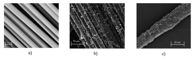
Fig. 4 (a) SEM image of untreated glass fibre roving ( $\times$ 2000); (b) SEM image graphene-based (coated) glass roving ( $\times$ 500); and (c) SEM image graphene-based (coated) glass roving ( $\times$ 1000).
