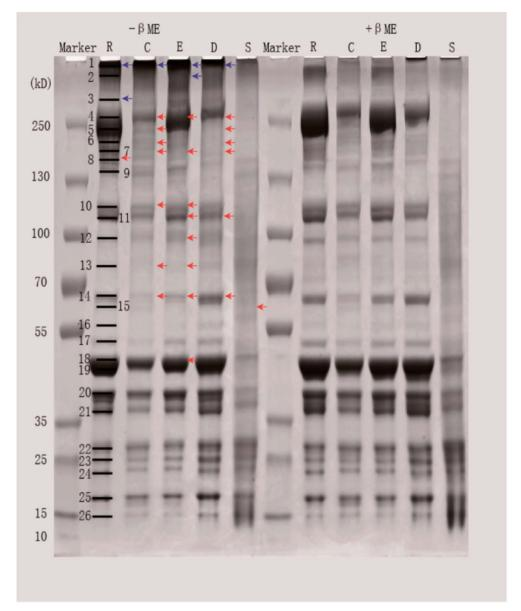
Fig. 2 SDS-PAGE patterns of proteins from different pork products. Samples were prepared without ( $-\beta$ ME) or with ( $+\beta$ ME) 5%  $\beta$ ME. Lanes R, C, E, D, and S represent raw pork, cooked pork, emulsion-type sausage, dry-cured pork, and stewed pork, respectively. Blue and red arrows represent decreased and increased intensities of lanes after treatment with 5%  $\beta$ ME, respectively.
