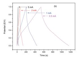
Fig. 12 Galvanostatic charge–discharge curves in 1.0 M  $\rm H_2SO_4$  for (a) GO and amine-functionalized GO at 1.0 mA cm $^{-2}$  and for (b) GO-DPA at different current densities.
