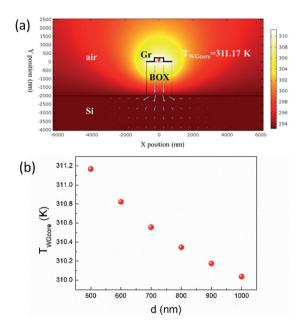
Fig. 6 (a) Thermal field distribution with 1.94  $\mu$ m-wide graphene nanoheater. Blue arrows shows directions of heat flux. (b) Waveguide core temperature as function of d.
