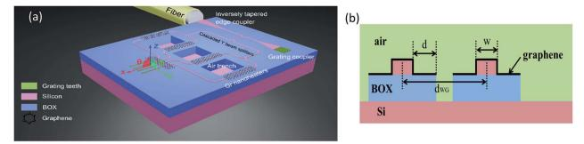
(a) Schematic of the proposed structure (not to scale). (b) Schematic cross-section of the phase-shifting region.
