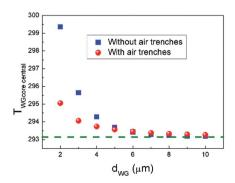
Fig. 12 Dependence of temperature at central waveguide core ( $T_{\rm WGcore\ central}$ ) on waveguide pitch ( $d_{\rm WG}$ ) with and without air trench. Dashed green line indicates the ambient temperature.
