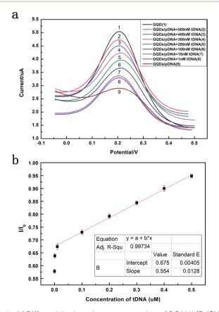
Fig. 6 (a) Differential pulse voltammograms plots of 0.2 M K<sub>3</sub>[Fe(CN)<sub>6</sub>] at pDNA (500 nM) immobilized GQDs modified GCE in 1.0 M KCl and that after hybridization with different concentrations of HBV-DNA (tDNA). (b) The plot of the peak current against the concentration of HBV-DNA.
