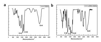
Fig. 4 FT-IR spectra of the GQDs (a) and pDNA-GQDs (b)
