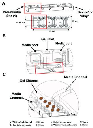
**Fig. 3** Microfluidic device. (A), The 3D cell culture chip (AIM Biotech) is shown with three independent microfluidic chambers per chip. Red rectangle identifies a single microfluidic chamber in the 3D cell culture chip. (B and C), Each device contains a center gel region with posts separating the gel region from the anti-parallel side channels. Gel loading port and media ports labeled (B), along with center and side channels (C).
