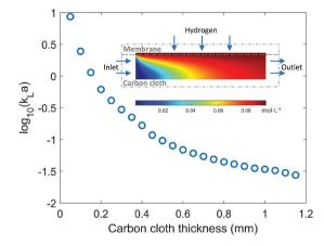
Fig. 3 The mass transfer coefficient  $k_L a$  values under various carbon cloth thicknesses. Insert figure: the hydrogen concentration profile in the membrane and carbon cloth (membrane thickness is 40  $\mu$ m, and carbon cloth thickness is 0.6 mm).
