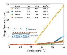
**Fig. 2** Required purge stream flowrates for various reaction temperatures and solvents. The inserted table shows the LELs in pure oxygen, boiling points (BP), and diffusion coefficients at 25 °C of the studied solvents.
