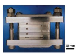
Fig. 5 (a) Cross-section of the inlet channels in a 3-layer stacked membrane reactor with blue arrows indicating the liquid flow and purple arrows indicating the gas flow. The outlet channels collect flow from each layer with reversed arrow directions. (b) Photo of a 3-layer stacked membrane reactor.
