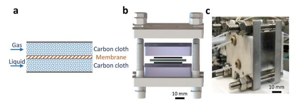
Fig. 1 (a) Gas-liquid membrane reactor schematics: Teflon AF membrane sandwiched between two sheets of carbon cloth layers to offer separation of gas and liquid while allowing the gas phase to diffuse through the membrane to react in the liquid phase. (b) Exploded-view CAD drawing of the gas-liquid membrane reactor. Two thin black layers are carbon cloth, and the thin blue layer is a Teflon AF membrane. (c) Photograph of assembled single-layer membrane reactor.
