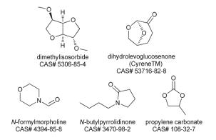
Fig. 3 Potential dipolar aprotic solvent replacements
